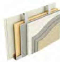
Type EC5i: Two layers of plasterboard, stud with glass wool between, sheathing board, EPS insulation, render
