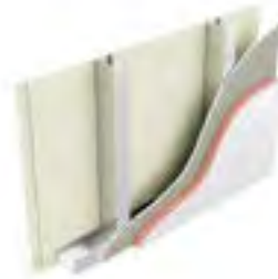
Type LE2: Two layers of plasterboard, stud, sheathing board, 50mm K15 Insulation
