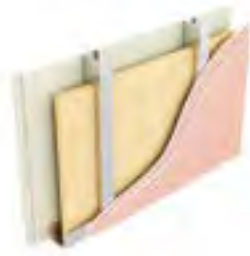
Type H2i: Two layers of plasterboard, stud with mineral wool between, two layers of plasterboard
