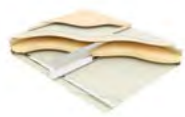
Type F3: Two layers of plasterboard, resilient bars, joists with mineral wool between, 15mm plywood, 19mm British Gypsum Plank, 53mm Danskin acoustic battens, 18mm V313 chipboard
