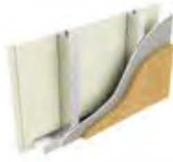
Type E4: Two layers of plasterboard, stud, sheathing board, 75mm Rockwool Duoslab Insulation
