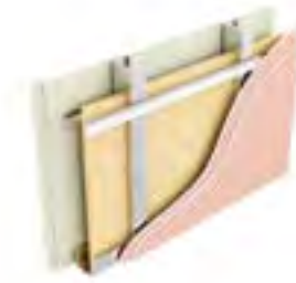
Type H4i: Two layers of plasterboard, resilient bar, stud with mineral wool between, resilient bar, two layers of plasterboard
