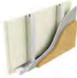
Type LE4: Two layers of plasterboard, stud, sheathing board, 75mm Rockwool Duoslab Insulation
