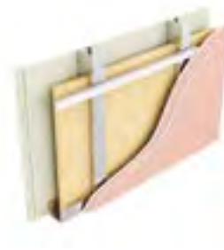
Type L3: Two layers of plasterboard, stud with mineral wool between, resilient bar, two layers of plasterboard
