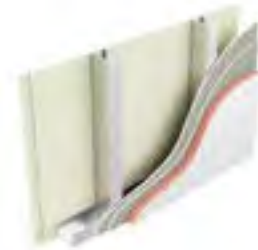
Type LE3: Two layers of plasterboard, stud, two layers of sheathing board, 50mm K15 Insulation
