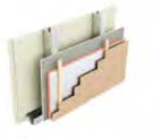
Type EC3: Two layers of plasterboard, stud, sheathing board, insulation, battens, timber cladding
