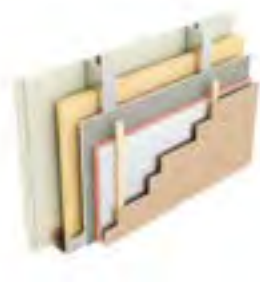
Type EC3i: Two layers of plasterboard, stud with mineral wool between, sheathing board, insulation, battens, timber cladding
