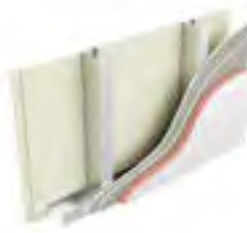
Type E3: Two layers of plasterboard, stud, two layers of sheathing board, 50mm K15 Insulation
