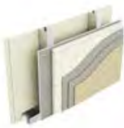
Type EC4: Two layers of plasterboard, stud, sheathing board, 20mm cavity, EPS insulation, render
