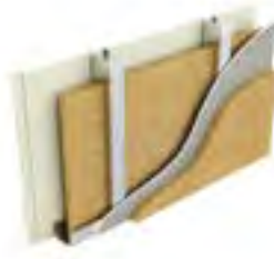
Type E4i: Two layers of plasterboard, stud with Rockwool between, sheathing board, 75mm Rockwool Duoslab Insulation
