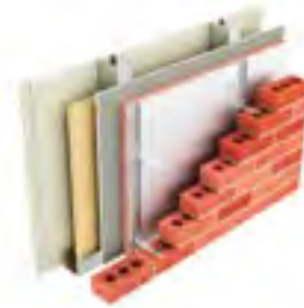
Type EC1i: Two layers of plasterboard, stud with mineral wool between, sheathing board, insulation, cavity, brickwork
