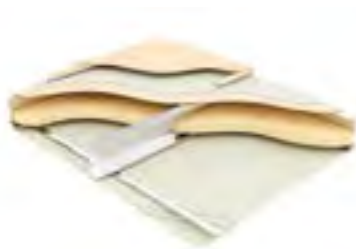
Type F9: Three layers of plasterboard, resilient bars, joists with mineral wool between, 15mm plywood, 19mm British Gypsum Plank, 70mm Collecta Deckfon acoustic battens, 18mm V313 chipboard
