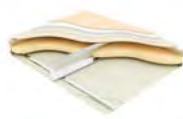
Type F2: Two layers of plasterboard, resilient bars, joists with mineral wool between, 15mm plywood, 19mm British Gypsum Plank, 8mm Cloud 9 Underlay, 12mm OSB
