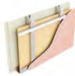
Type H3i: Two layers of plasterboard, stud with mineral wool between, resilient bar, two layers of plasterboard
