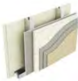
Type EC5: Two layers of plasterboard, stud, sheathing board, EPS insulation, render
