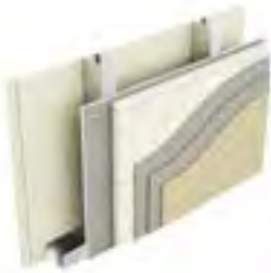
Type EC4: Two layers of plasterboard, stud, sheathing board, 20mm cavity, EPS insulation, render
