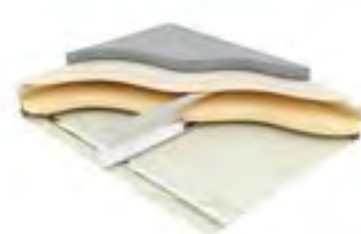
Type F8: Two layers of plasterboard, resilient bars, joists with mineral wool between, 15mm plywood, 19mm British Gypsum Plank, Collecta Screedboard 28
