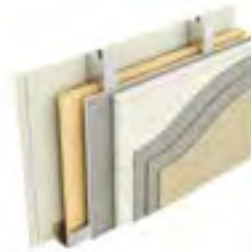
Type EC4i: Two layers of plasterboard, stud with glass wool between, sheathing board, 20mm cavity, EPS insulation, render
