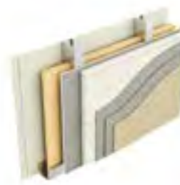
Type EC4i: Two layers of plasterboard, stud with glass wool between, sheathing board, 20mm cavity, EPS insulation, render
