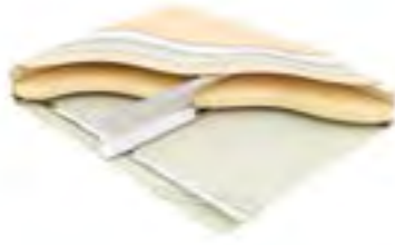
Type F5: Three layers of plasterboard, resilient bars, joists with mineral wool between, 15mm plywood, 19mm British Gypsum Plank, 8mm Cloud 9 Underlay, 12mm OSB
