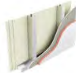
Type LE6: Three layers of plasterboard, stud, sheathing board, 50mm K15 Insulation
