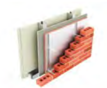
Type EC1: Two layers of plasterboard, stud, sheathing board, insulation, cavity, brickwork
