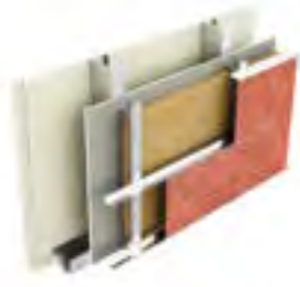
Type EC2: Two layers of plasterboard, stud, sheathing board, insulation, ventilated rainscreen
