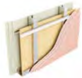
Type L8: Three layers of plasterboard, resilient bar, stud with mineral wool between, resilient bar, three layers of plasterboard
