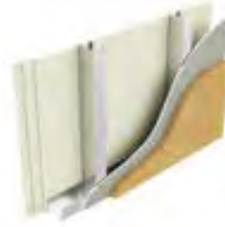
Type LE8: Three layers of plasterboard, stud, sheathing board, 75mm Rockwool Duoslab Insulation
