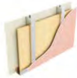
Type H1i: Layer of plasterboard, stud with mineral wool between, layer of plasterboard
