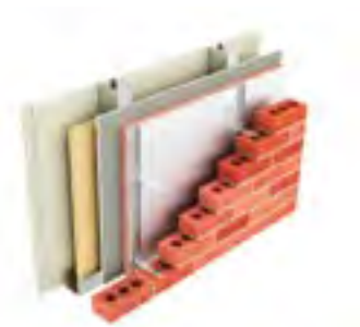
Type EC1i: Two layers of plasterboard, stud with mineral wool between, sheathing board, insulation, cavity, brickwork
