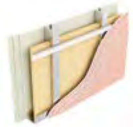
Type L7: Three layers of plasterboard, stud with mineral wool between, resilient bar, three layers of plasterboard
