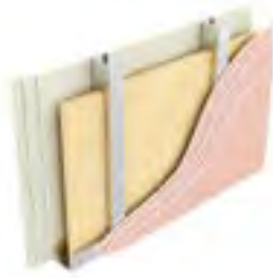
Type L6: Three layers of plasterboard, stud with mineral wool between, three layers of plasterboard
