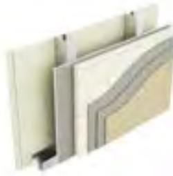
Type EC5: Two layers of plasterboard, stud, sheathing board, EPS insulation, render
