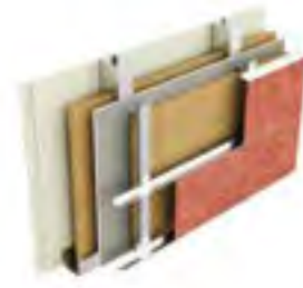
Type EC2i: Two layers of plasterboard, stud with mineral wool between, sheathing board, insulation, ventilated rainscreen
