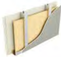
Type E1i: Two layers of plasterboard, stud with mineral wool between, sheathing board
