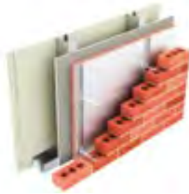
Type EC1: Two layers of plasterboard, stud, sheathing board, insulation, cavity, brickwork
