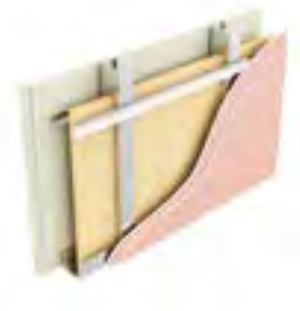
Type L4: Two layers of plasterboard, resilient bar, stud with mineral wool between, resilient bar, two layers of plasterboard
